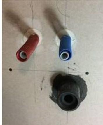
Typical sample of penetrating services with gap widths between 10 and 30mm
