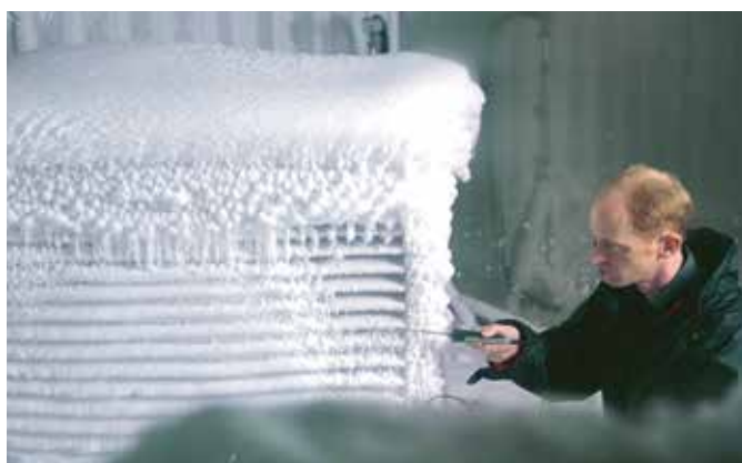
Climatic chambers simulate all possible operating conditions
